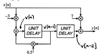
(a) Write a simple formula for the difference equation defined by the signal flow graph. Since this is not a standard form, you must write the equations for signals at each node of the signal flow graph.
