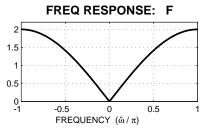
For each of the frequency response plots (A, B, C, D, E, F), determine which one of the following systems (specified by either an H(z) or a difference equation) matches the frequency response (magnitude only). NOTE: frequency axis is **normalized**; it is  $\hat{\omega}/\pi$ .
