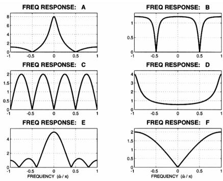
For each of the frequency response plots (A, B, C, D, E, F), determine which one of the following systems (specified by either an H(z) or a difference equation) matches the frequency response (magnitude only). NOTE: frequency axis is **normalized**; it is  $\hat{\omega}/\pi$ .
