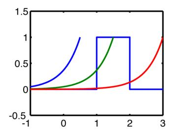
We have three cases, illustrated by the figure above. We choose to flip the input, and not h(t). In the first case, t < 1, there is no overlap between between  $h(\tau)$  and  $x(\tau - t)$ . In the second and third cases, 1 < t, there is overlap. In the third case, the overlap ends at  $\tau = 2$ . We generated the above plot using the following MATLAB commands:
