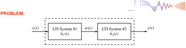
In the cascade of two LTI systems shown in the figure above, the first system has an impulse response
