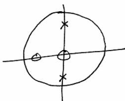
$$S_4: H(z) = \frac{1 + \frac{3}{4} z^{-1} - \frac{1}{4} z^{-2}}{1} = \frac{z^2 + \frac{3}{4} z - \frac{1}{4}}{z^2} = \frac{(z + 1)(z - \frac{1}{4})}{(z)(z)}$$
