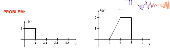
Consider the input signal x(t) and the impulse response h(t) shown above. The output of an LTI system is  $y(t) = x(t) * h(t) = \int_{-\infty}^{\infty} x(\tau)h(t-\tau)d\tau$ .
